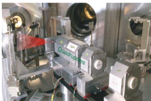
SAPHIR beam transport setup of the laser-produced plasma proton beam for radiobiology at high dose.
